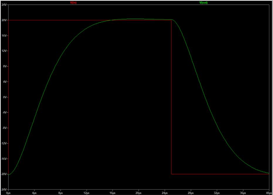
As you can see, the slew is limited to **4 V/μS** by the output filter. But exactly, how much voltage can we deliver before the signal is distorted?
