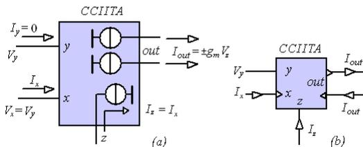
Fig. 4. CCIITA - a) behavior schematic description b) schematic symbol
