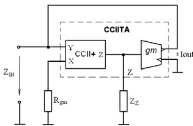
Fig. 5. Imittance inverter built from CCIITA
