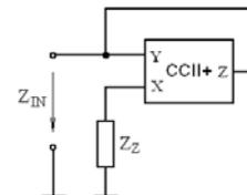
Fig. 8. Negative imittance converter from one CCII+
