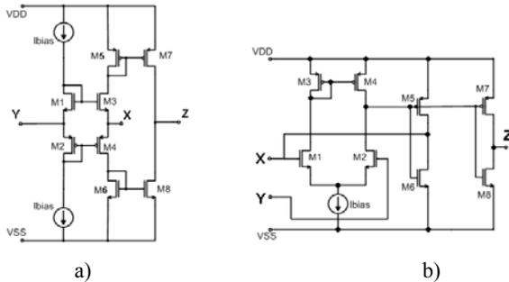
Fig. 9. Internal topology of current conveyor CCII+
