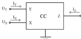
Fig. 1. Current Conveyor schematic symbol
