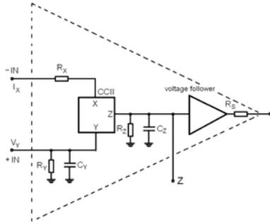
Fig. 2. Block realization of transimpedance amplifier CFA
