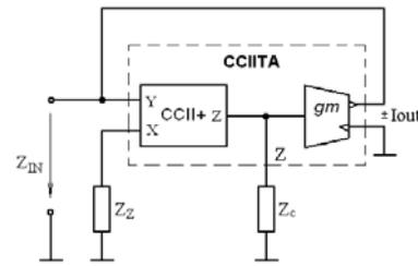
Fig. 6. Positive imittance converter built from CCIITA
