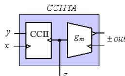
Fig. 3. Block internal schematic of the CCIITA
