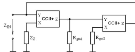
Fig. 7. Negative imittance converter built from two CCII+
